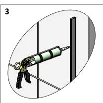
RUN A SMALL BEAD OF SILICONE DOWN THE INSIDE OF THE WALL PROFILES BEFORE FITTING GLASS. NOW SLIDE THE GLASS PANELS (ITEM 2) INTO THE PROFILES.
