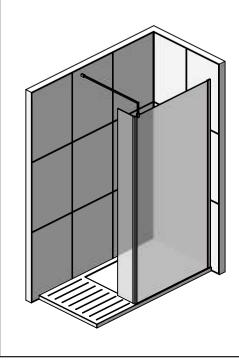
SLIDE THE RETURN GLASS PANEL (ITEM 16) INTO THE CORNER PROFILE (ITEM 15) ENSURING ITS FULLY INSIDE.
