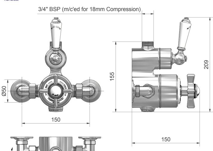
Supply connections are 15mm compression, and can be swivelled for top, bottom or through wall feed. Hot is on left, cold is on the right (viewed from front).
