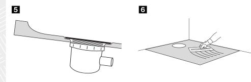
Fit the waste unit to the shower tray following the instructions supplied with the unit and protect exposed threads with masking tape. Before proceeding dry fit all items in-situ to ensure compatibility and then screw the plywood level into position.
