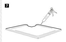
Before fitting, apply copious amounts of silicone to the edges of the shower tray **(\Odd)** against all wall contact points.
