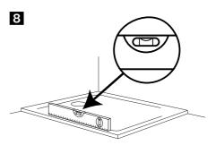
Place the shower tray **①** onto the wet adhesive ensuring that it is fully supported by the mix. Check the level of the top rims only as the shower tray has a built in fall for adequate drainage.
