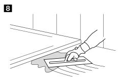
When the adhesive has set, remove any excess mix and masking tape, then make connection between the shower tray and waste piping. The shower tray and all connections MUST now be checked for water tightness, flow and adequate drainage over the entire area.
