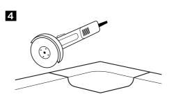
Carefully cut the marked area from the shower tray using a minimum of a four inch (approx 102mm) diamond blade (suitable for cutting stone) on an angle grinder or other suitable cutting tool.
