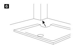
Test fit the shower tray in-situ making any further adjustments as necessary to ensure a snug fit.
