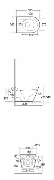
Dimensions: All dimensions in mm. Tolerance of vitreous china & fireclay items:  $\pm$  5% for below 200mm and  $\pm$  3% for above 200mm; for all other items tolerance  $\pm$  1%. Note: Due to a continuing development program to improve design and performance, the manufacturer reserves all rights to vary specifications without prior information. Please note accessories are for photographic use only.
