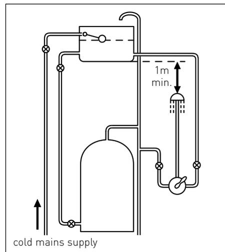
**⚠ Important:** If you install this shower valve with a gravity fed system, there must be a minimum head (vertical distance) from the underside of the cold water storage tank to the outlet of at least 1 metre.
