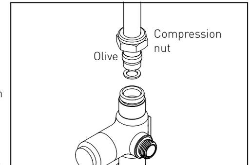
3. Push the arm into the top bracket, ensuring the nut and olive are fitted to the arm. Tighten the nut fully using a suitable spanner.
