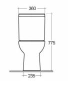
Dimensions: All dimensions in mm. Tolerance of vitreous china & fireclay items: ± 5% for below 200mm and ± 3% for above 200mm; for all other items tolerance ± 1%. Note: Due to a continuing development program to improve design and performance, the manufacturer reserves all rights to vary specifications without prior information. Please note accessories are for photographic use only.
