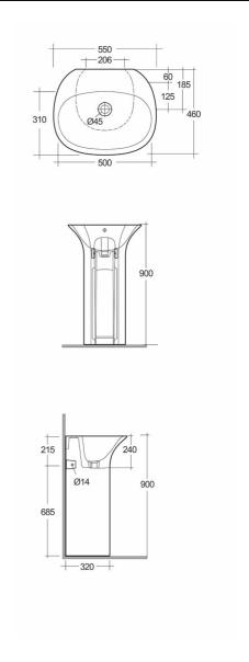
Dimensions: All dimensions in mm. Tolerance of vitreous china & fireclay items:  $\pm$  5% for below 200mm and  $\pm$  3% for above 200mm; for all other items tolerance  $\pm$  1%. Note: Due to a continuing development program to improve design and performance, the manufacturer reserves all rights to vary specifications without prior information. Please note accessories are for photographic use only.
