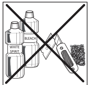
Step J Applying Silicone Sealant And Cleaning Seal from the top of the wall channel to the bottom on the INSIDE and Outside between the wall channel and the wall, and between the bottom profile and shower tray as shown. Wash down with clean warm water and a soft clean cloth or sponge. Please do not use bleach, alkaline or acid-based, aggressive or abrasive cleaning products.
