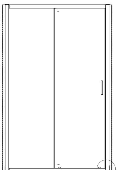
EXTERNALLY SILICONE SEAL THE WALL PROFILES WHERE THEY MEET THE WALL AND THE BOTTOM PROFILE WHERE IT MEETS THE TRAY. ALL IN A CONTINUOUS BEAD.
