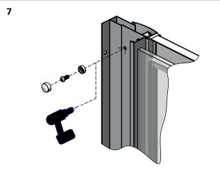
WHEN THE FRAME IS READY TO BE FIXED, DRILL THROUGH THE HOLES IN ITEMS 2 & 5 WITH A 3mm DRILL BIT.
