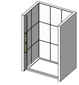
MAKE SURE THE WALL PROFILES ARE TRUE AND SQUARE WITH A SPIRIT LEVEL. MARK THROUGH THE FIXING HOLES WITH A PENCIL. REMOVE PROFILES, DRILL AND PLUG THE WALLS (ITEM 25). THE WALL PLUGS SUPPLIED MAY NOT BE SUITABLE FOR YOUR SUBSTRATE, USE SUITABLE FIXINGS. NOW REFIT ONE WALL PROFILE IN PLACE USING ITEM 21, 22 & 23.
