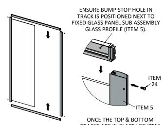
SLIDE THE TOP & BOTTOM TRACKS INTO THE GLASS PROFILE AND MAGNETIC PROFILE UNTIL FLUSH.
